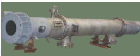
GACL :- Sessate Recovery Column As Per ASME Sec VIII Code-1, 2015
