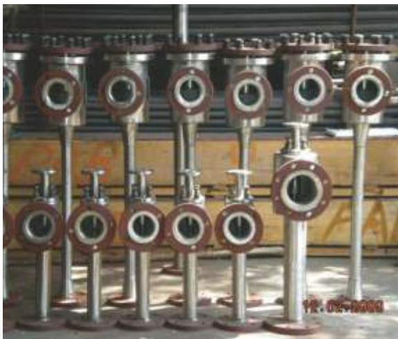
Steam jet + Liquid Jet Ejector Combination System (1.0 torr)
