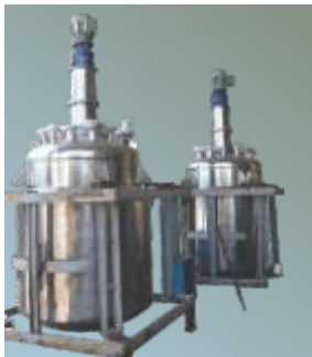
GMP Reactor 2 Kl With Hot & Cold Insulation:- Adroit Pharmachem Pvt Ltd.
