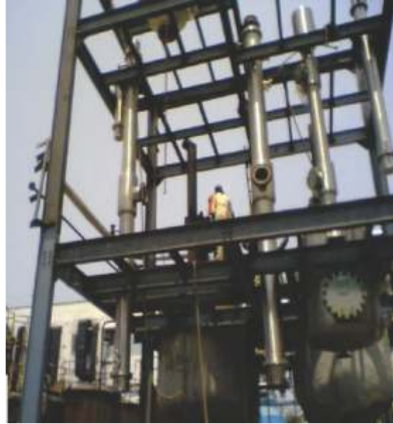
Multi Effect Evaporators (ss-316)
