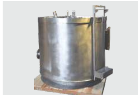
Milk Process Spray Drying - Air Dispaser (12 Tons For Day)
