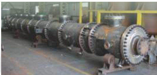
GACL:-DHA Stripper Column Under Third Party:- PDIL,100% Radiography, EPC :- L & T Chiyoda
