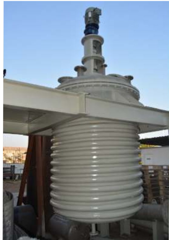
Gland Type, Limpet Type, Reactor
