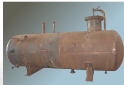
GACL:-DHA Stripper Drain Tank Under Third Party:- PDIL,100% Radiography, EPC:- L & T Chiyoda
